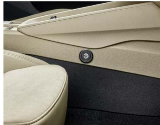
**Mechanical transmission locking system**
