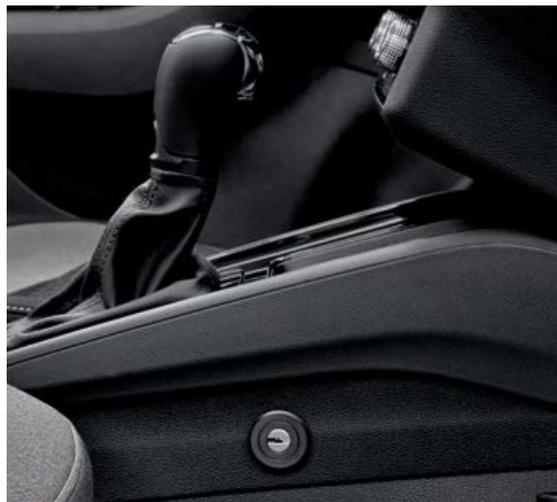
**Mechanical gearbox locking system**
