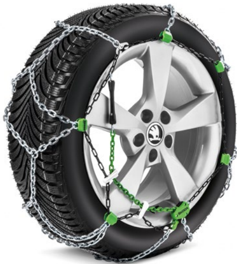
Snow chains for wheels 15" 195/65 R15 000 091 387AQ | for wheels 16" 195/60 R16
