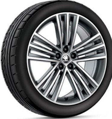
SIRIUS 654 071 498F HA7 light-alloy wheel 7.0J × 18" ET39 for 205/45 R18 anthracite metallic brushed
