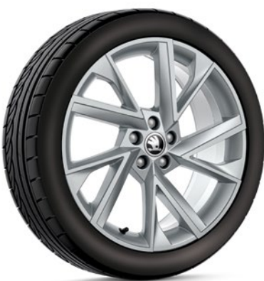
VEGA 654 071 498H 8Z8 light-alloy wheel 7.0J × 18" ET39 for 205/45 R18 silver metallic
