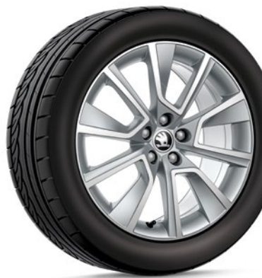
BRAGA 654 071 497L 8Z8 light-alloy wheel 6.5J × 17" ET40 for 205/50 R17 silver metallic
