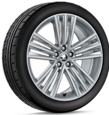
SIRIUS 654 071 498M 8Z8 light-alloy wheel 7.0J × 18" ET39 for 205/45 R18 silver metallic
